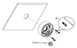
④ Mount the rubber plug to the gap of the mounting base and fasten the camera onto the mounting base.
