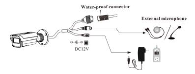
\* It is recommended to install the water-proof connector for outdoor installations.
